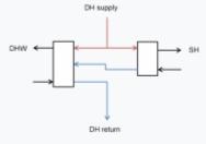
Figure 5. Simplified schemes of 2-step connection of domestic hot water and space heating.
