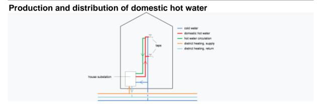
Figure 1. Sketch of a typical domestic water installation. The incoming cold water is lead to the taps and to the house substation. In the case of hot-water circulation, the DHW is circulated back to the substation in order to maintain a high between tapings to reduce waiting time.
