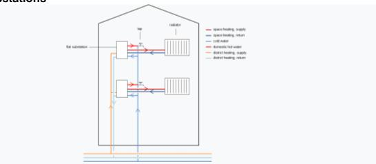
Figure 3. Sketch for DHW and SH system in a building with flat substations. Only one tap and one radiator per flat are shown; in a real building the system is obviously more branched. The heat exchange to the local DHW and SH systems occur in every flat and no hot-water circulation is needed.
