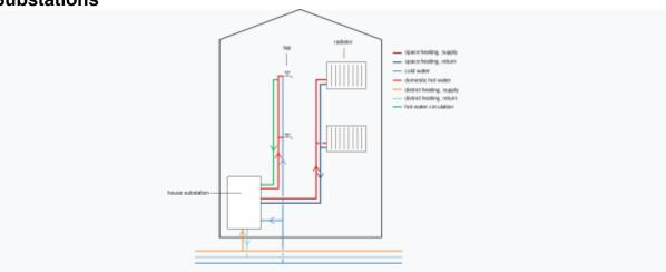
Figure 2. Sketch for traditional SH and DHW systems in a building. The DHW and the SH are produced centrally in the building and the hot-water circulation is used to guarantee that the DHW is supplied within a reasonable time for the taps far away from the house substation.
