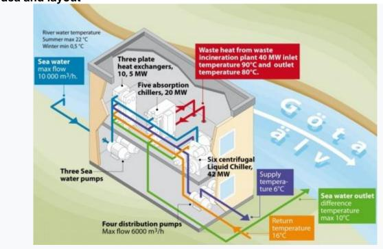
Schematic illustration of free cooling with river water in Gothenburg[1]
