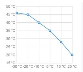
Figure 3: Mapping of the forward temperature in relation to the outdoor temperature
