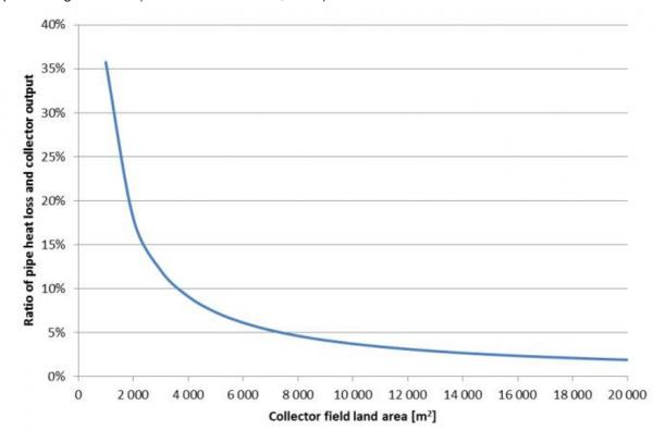
Pipe heat loss per km distance between collector field and district heating network connection point related to collector output for varying land area size
