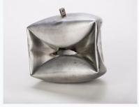
Damages to a float gauge caused by a Joukowski pressure peak. Photo by CEphoto, Uwe Aranas (<u>link</u>)(<u>CC BY-SA-3.0</u>).
