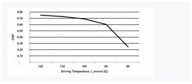
Figure 5 Relationship between COP for an absorption cooler and temperature of the heat source
