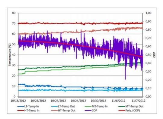
Figure 1 Different supply and return temperature for the district heating run by absorption cooler
