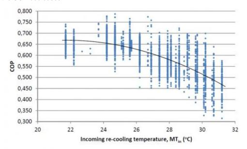
Figure 3 Relationship between COP for the absorption cooler and the recooling temperature
