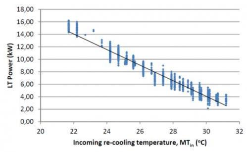
Figure 2 Relationship between power for the absorption cooler and the recooling temperature
