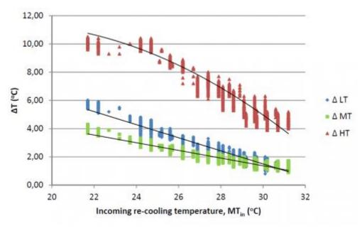
Figure 4 Relationship between delta temperature for the absorption cooler and the re-cooling temperature
