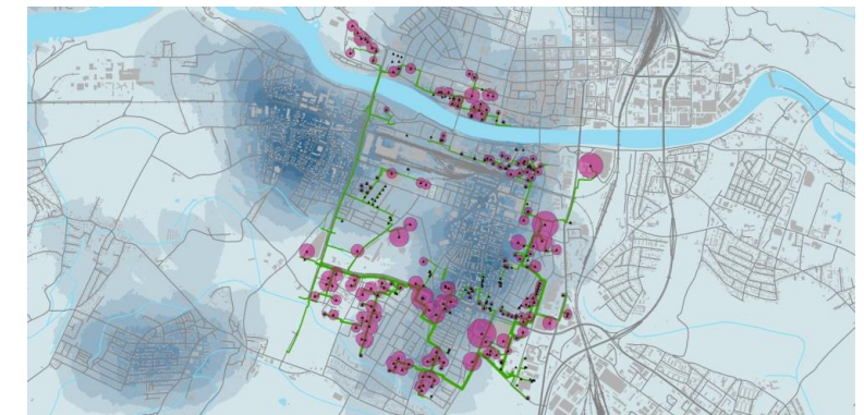
PM10 emissions (individual biomass boilers)
