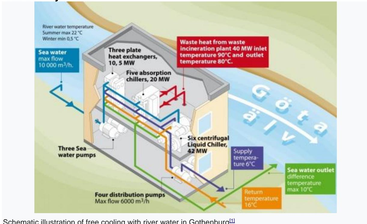
Schematic illustration of free cooling with river water in Gothenburg<sup>[1]</sup>
