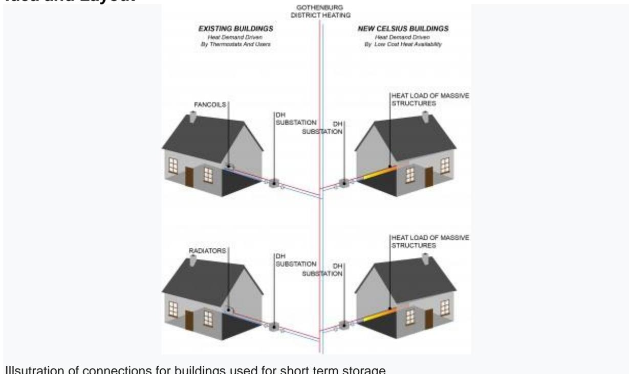
Illustration of connections for buildings used for short term storage
