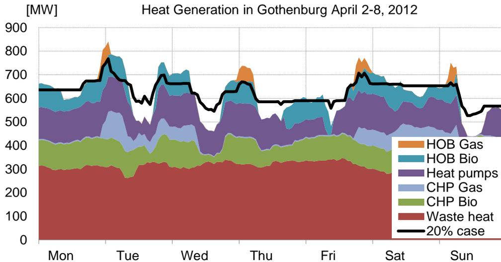
**Fig. 11** Example of the heat generation in Gothenburg during one week with a possible load curve from the 20% case as an overlay.
