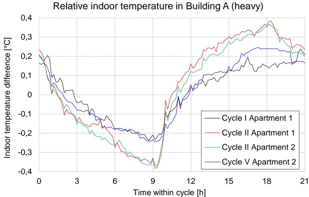
**Fig. 6** Indoor temperature variations caused by the pilot test. Each curve is based on average values over a period of four to six weeks.
