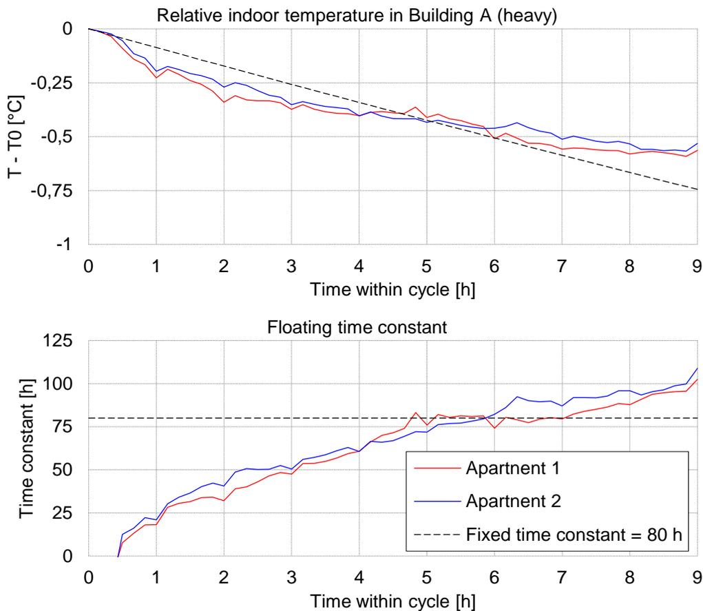
**Fig. 7** Top graph: Average indoor temperature profile during DP. The *fixed time constant* has a slightly rising concave shape. Bottom graph: *floating time constant* based on the temperature profile from the top graph.
