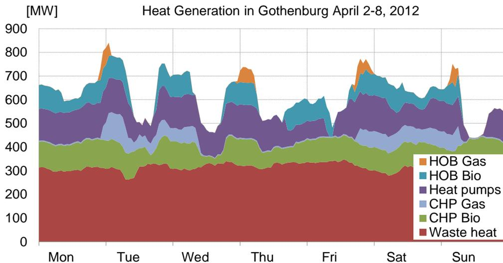
**Fig. 1** Example of the heat generation in Gothenburg during one week. A total of 28 different heat sources (boilers, heat pumps, waste heat sources, etc.) are grouped into six categories. During this week, heat sources were started and stopped a total of 36 times.
