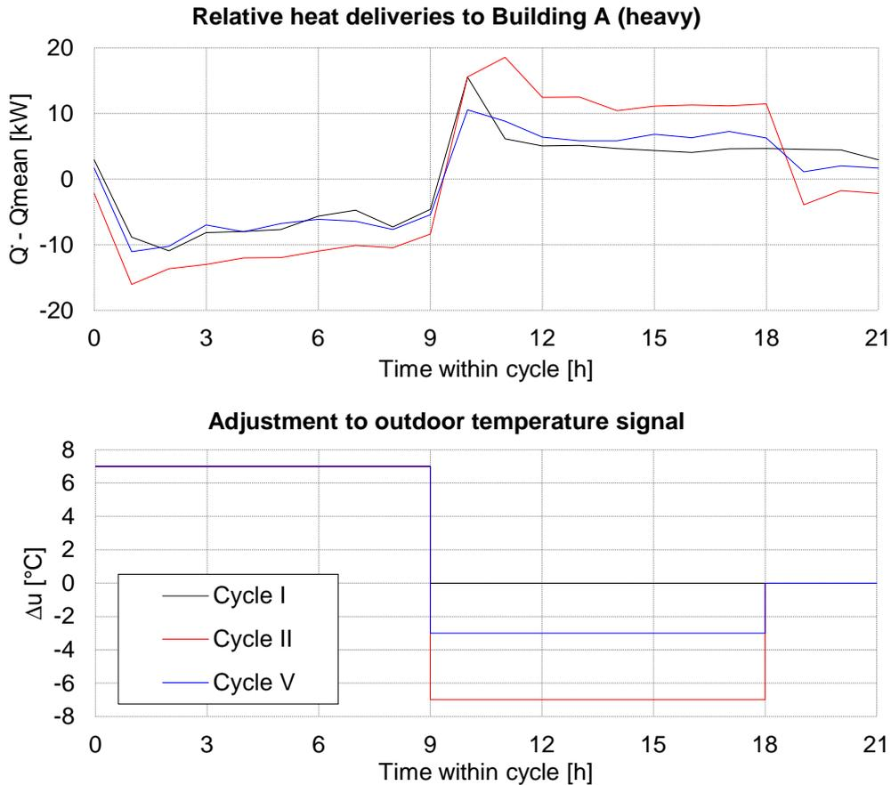
**Fig. 5** Heat delivery profiles relative to the control cycle average for Building A. Each profile is based on five to eight weeks of measurements.
