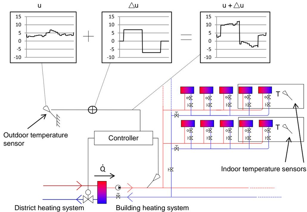
**Fig. 3** Schematic of how the control was implemented in the pilot test.
