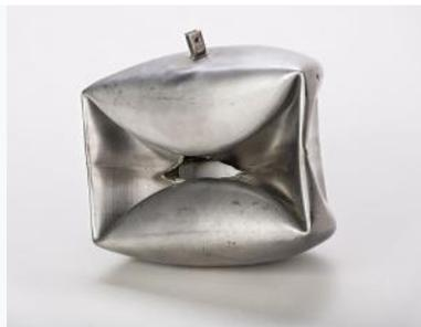
Damages to a float gauge caused by a Joukowski pressure peak. Photo by CEphoto, Uwe Aranas ([link](#))(CC BY-SA-3.0).
