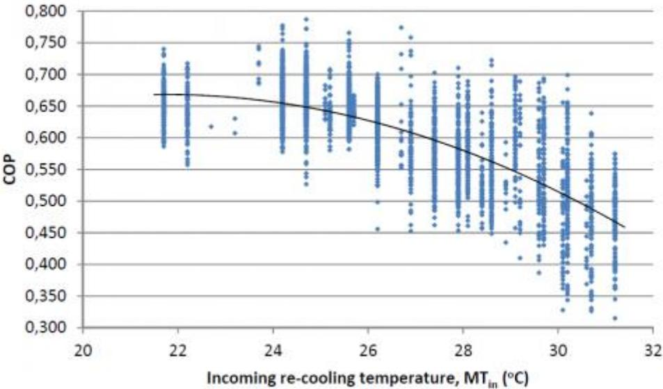
Figure 3 Relationship between COP for the absorption cooler and the recooling temperature
