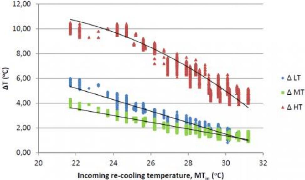
Figure 4 Relationship between delta temperature for the absorption cooler and the re-cooling temperature
