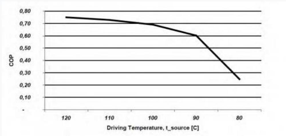
Figure 5 Relationship between COP for an absorption cooler and temperature of the heat source
