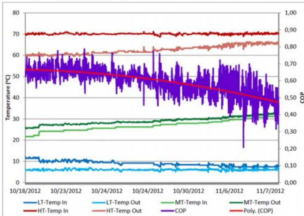
Figure 1 Different supply and return temperature for the district heating run by absorption cooler
