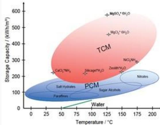
Storage capacity vs temperature for sensible, latent and thermochemical TES
