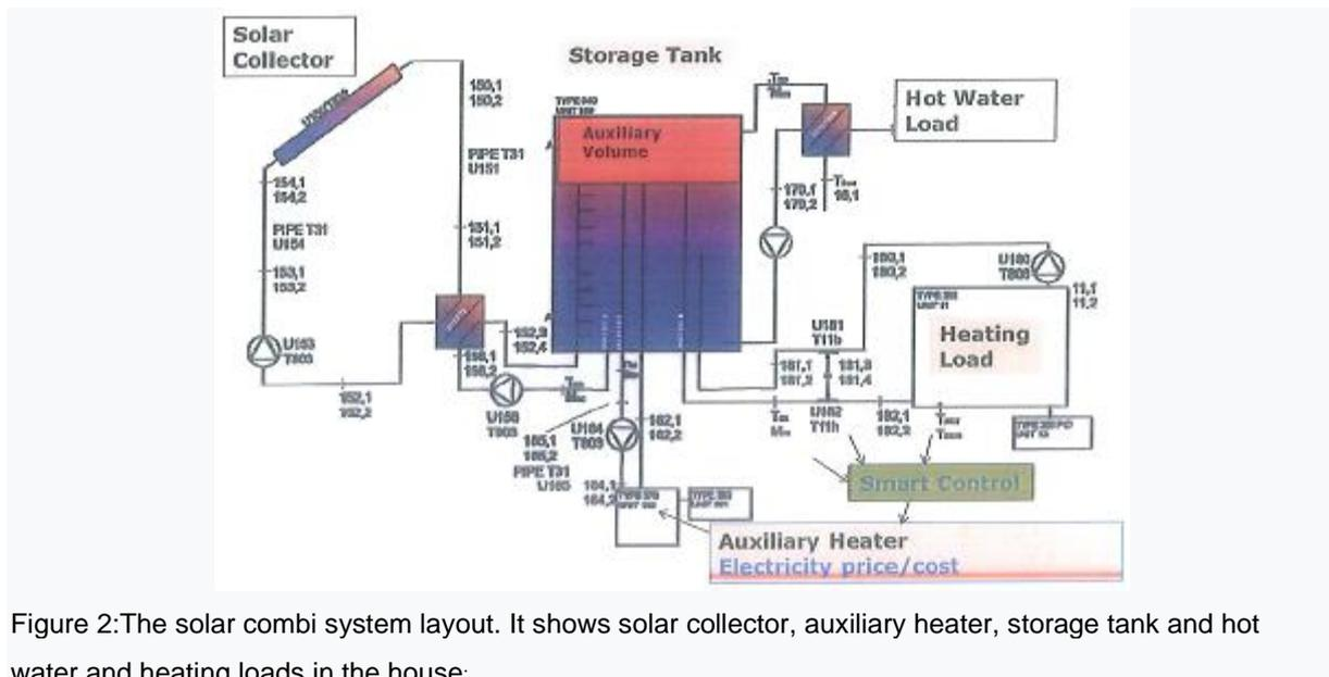
Figure 2: The solar combi system layout. It shows solar collector, auxiliary heater, storage tank and hot water and heating loads in the house
